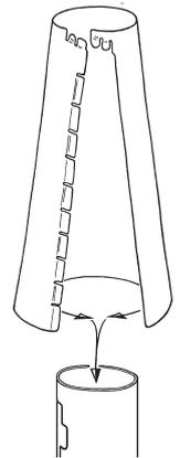
the chimney through the opening in the tent and put it onto the lower part. If your tent is very high you will have to secure your chimney onto the tent pole with a wire rope. Now your stove is ready to start a fire.
